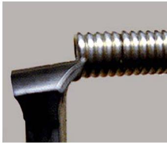
**3.** Use your flush cutter - cut the end tip flush with the rest of the coil.
